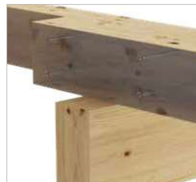
Joint between two passing-by beams
