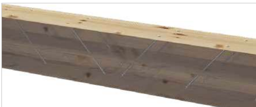
Reinforcement by coupling of beams
