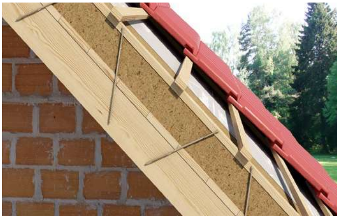
Fixing of soft over-rafter insulation
