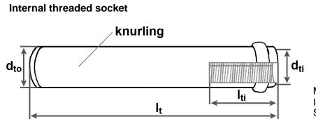
Marking: Identifying mark of the producer "m" Size of internal thread e.g. M8
