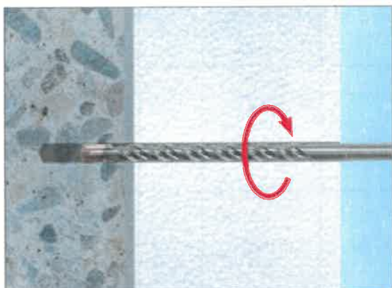
1. Drill hole by corresponding drilling method
