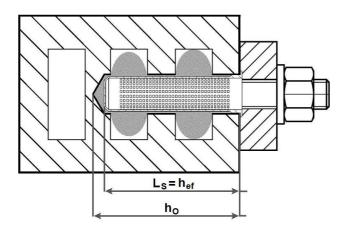
Installation of internal threaded socket with sieve
