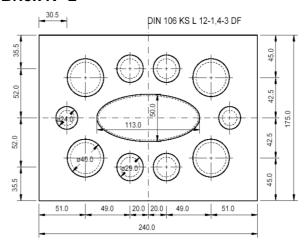
Hollow sand lime brick KSL 12-1,4-3DF according to EN 771-2 length/width/height = 240 mm/175 mm/113 mm  $f_b \geq$  12 N/mm² /  $\rho \geq$  1,4 kg/dm³
