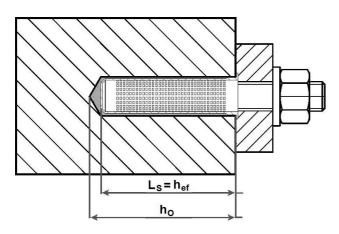
Installation of internal threaded socket with sieve
