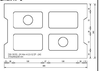
Concrete masonry unit Hbn 4-12DF according to EN 771-3 length/width/height = 370 mm/240 mm/238 mm  $f_b \ge 4 \text{ N/mm}^2 / \rho \ge 1,2 \text{ kg/dm}^3$
