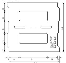
Lightweight concrete hollow block HbI 4-0,7-8DF according to EN 771-3 length/width/height = 250 mm/240 mm/248 mm  $f_b \geq 4,0 \ N/mm^2 \ / \ \rho \geq 0,7 \ kg/dm^3$
