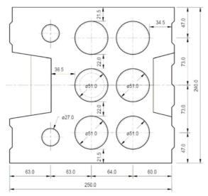
Hollow sand lime brick KSL 12-1,4-8DF according to EN 771-2 length/width/height = 250 mm/240 mm/237 mm  $f_b \geq 12 \ N/mm^2/\ \rho \geq 1,4 \ kg/dm^3$
