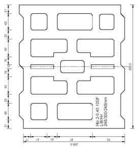
Lightweight concrete hollow block HbI 2-0,45-10DF according to EN 771-3 length/width/height = 250 mm/300 mm/248 mm  $f_b \ge 2,0 \text{ N/mm}^2$  /  $\rho \ge 0,45 \text{ kg/dm}^3$
