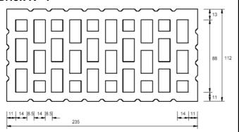
Hollow clay brick HLz 12-1,0-2DF according to EN 771-1 length/width/height = 235 mm/112 mm/115 mm  $f_b \ge 12 \text{ N/mm}^2 / \rho \ge 1,0 \text{ kg/dm}^3$
